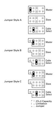
**Figure 6. Jumper Positions**
