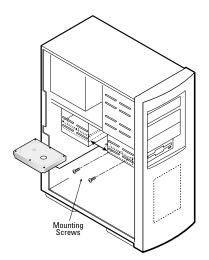
Figure 7. Typical 3.5-inch Device Bay Installation
