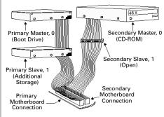
Figure 11. Typical Device Configuration
