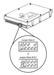
Figure 5. Determine Jumper Style
