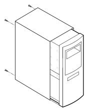
Figure 3. Removing the System Cover
